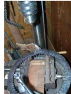
Drilling the rivet holes
